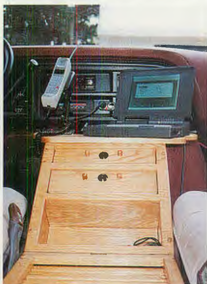
Laptop computer station atop Anderson's handmade between-seats storage console is fax-capable, features cellular phone and can access numerous intelligence databases.
